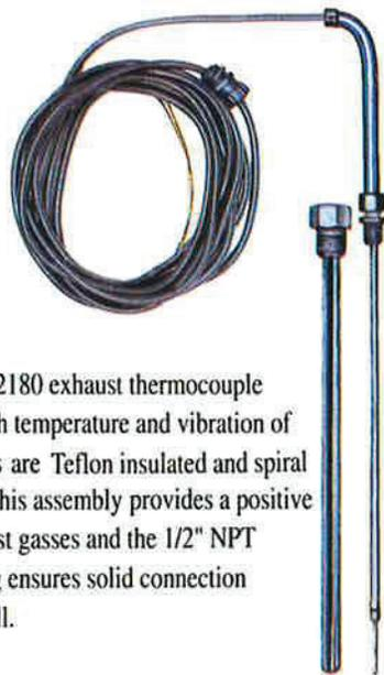
The PYCO 02-2180 exhaust thermocouple holds up to the high temperature and vibration of gas turbines. Wires are Teflon insulated and spiral armor protected. This assembly provides a positive seal against exhaust gasses and the 1/2" NPT compression fitting ensures solid connection with the thermowell.
