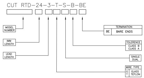
THE CUTTABLE RTD SENSOR IS USED WHEN YOU PREFER TO BUY SINGLE LENGTH RTD SENSORS FOR MULTIPLE LENGTH APPLICATIONS. IDEAL FOR USE IN THE FIELD WHERE THE EXACT LENGTH MAY NOT BE KNOWN. THEY ARE CUT WITH A TUBE CUTTER BY THE END USER ONCE THE REQUIRED LENGTH IS DETERMINED. IT CAN BE USED WITH MULTIPLE ACCESSORIES TO MEET YOUR APPLICATION NEEDS.
