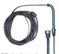
The PYCO 02-2180 exhaust thermocouple holds up to the high temperature and vibration of gas turbines. Wires are Teflon insulated and spiral armor protected. This assembly provides a positive seal against exhaust gasses and the 1/2" NPT compression fitting ensures solid connection with the thermowell.
